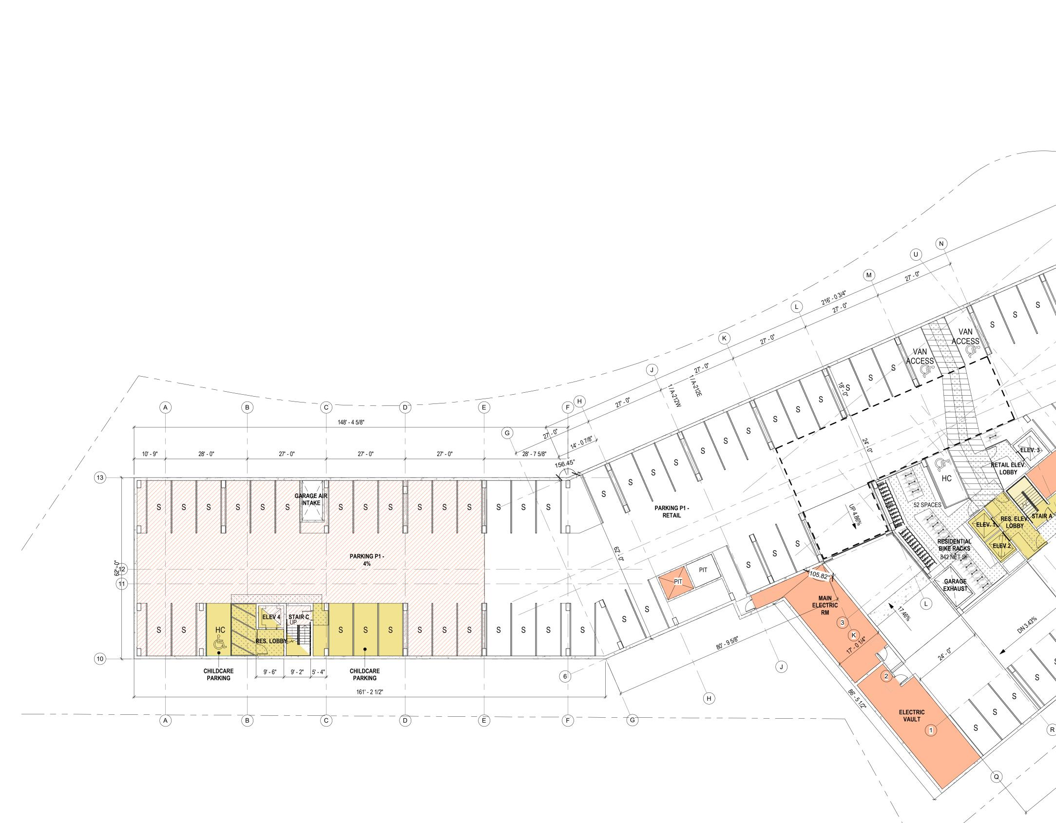
1 LEVEL P1 FLOOR PLAN A-202 SCALE: 1/16" = 1'-0"
